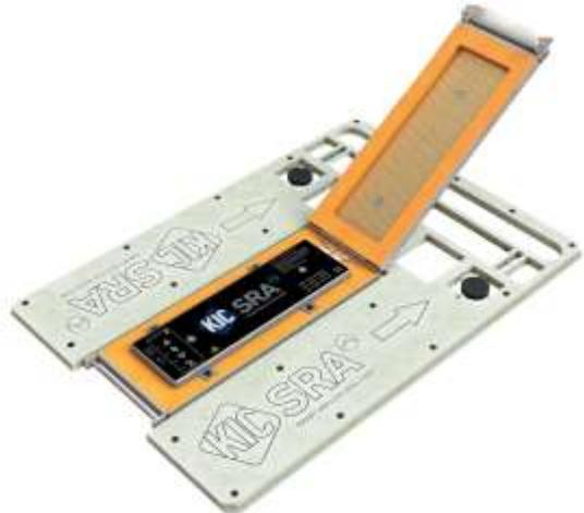
As it contains a built-in data collection module, the SRA is an all-in-one smart fixture. This means that the SRA can be used independently no matter whose profiler you may currently have. The SRA is an integrated fixture and profiler specifically designed for collecting reflow oven related data to analyze and track machine stability from run to run, and over time.
