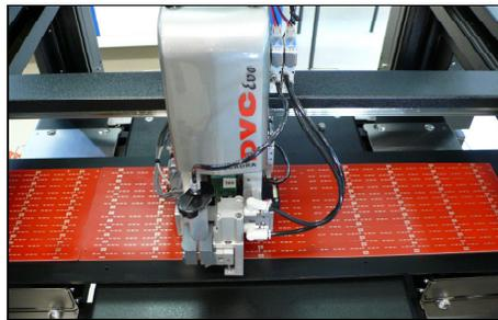
The **conveyor** is a simple and effective tool that **allows to place components on large pcbs**. To cover the needs of many applications, the system can be provided in four configurations, with working plates of different sizes (850x200mm, 850x350mm, 850x420mm and **1200x200mm**), suitable for a wide range of boards/panels.
