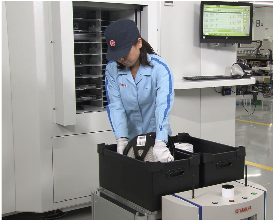
Photo 1: Delivery of components from the SMD storage system and transfer using AGV
