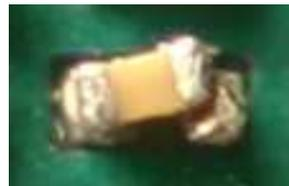
Fig5. Skewed component due to inaccurate placement
