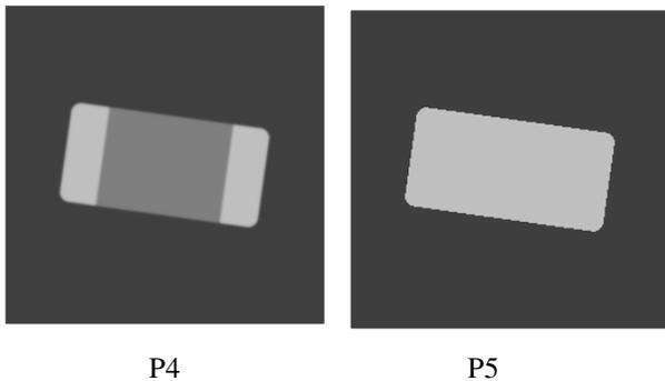
**Figure 2.** P4 represents a simplified image of a chip capacitor on a black background. P5 represents the resultant blob after the image of the chip is separated from the background.
