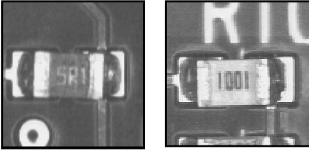
**Figure 5.** Two examples of chip resistors that would induce false failures due to variation in body color.
