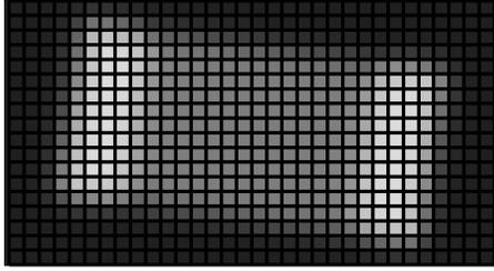
In the two images above, the same component appears in the same region of interest but with a slightly different angle. Using pixel-by-pixel “grey scale” comparison, the second image should fail [3], due to lack of information at certain pixel locations within the region of interest. As you can see, this methodology has very poor accuracy when a component is skewed.
