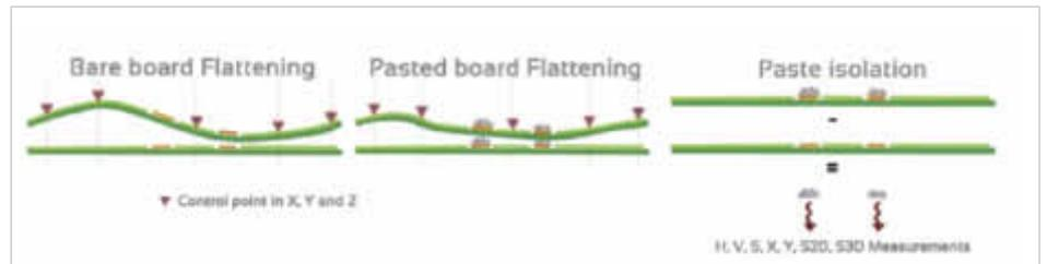
**PCB warpage compensation:** As can be seen above Pi identifies multiple reference points in X, Y and Z. Pi uses these references to overcome stretch and also to determine the appropriate zero height for each pad, regardless of which layer the pad is located on. This ensures that Pi measures a true reference height and thus a true volume of the solder deposit
