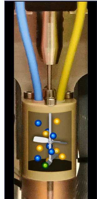
**Figure 4 – Dynamic (or active) mixing consists of an "impeller" or a "blade" that mixes the two parts within a chamber as the material is flowing by.**
