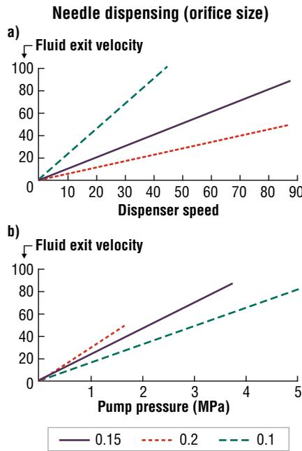
**Figure 2.** Plots of orifice size of a needle dispenser vs. the fluid exit velocity showing that **a)** a 0.15mm needle matches the dispense speed; and **b)** high pressures are required for dispensing over 40mm/sec with 0.15mm orifice and a 0.1mm orifice.
