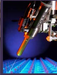
LED assembly includes dispensing of various materials, such as yellow phosphor filled silicone. Typical dispensing applications are:
