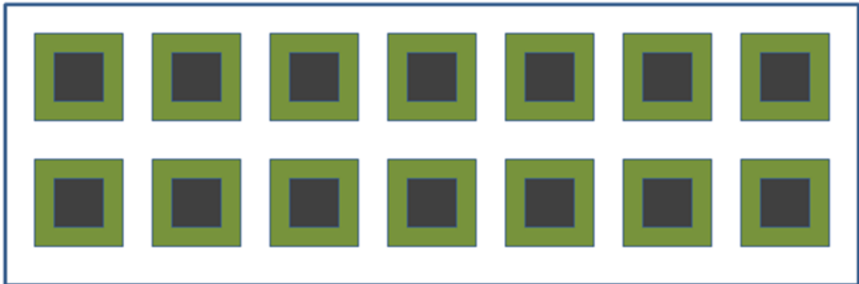
Figure 1: 2 x 7 Boat Die Layout for Traditional Flip Chip
