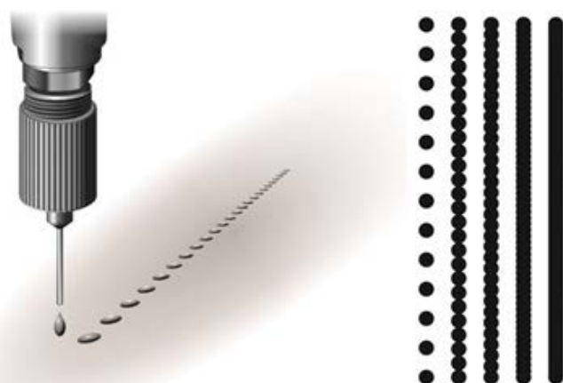
Figure 3. Jet applicator with needle extension. Tip and coating pattern (left), top view of possible patterns (right).
