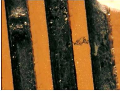
**Figure 9.** Dendrites Growth on Paste B boards under Customized #3 ECM Test
