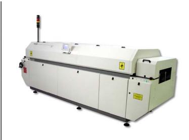
The IR/convection cure module is ideal for mid- to high-volume production. The oven features precise control of conveyor speed and internal thermal environment. Infrared panels and exclusive heat dispersion plates transfer heat by convection.
