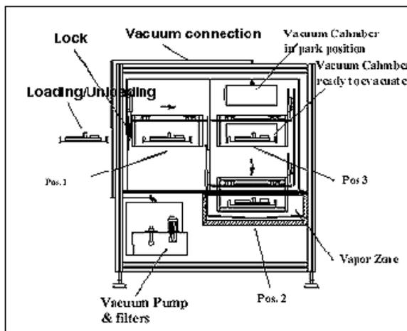
**Figure 3.** Sketch - condensation reflow system with vacuum chamber
