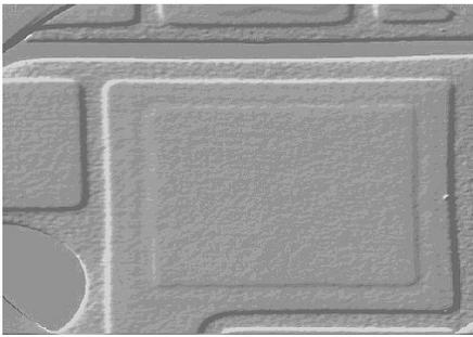
**Figure 2.** Soldered joint after vacuum treatment
